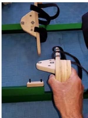
The foot has a wooden heel and a row of single slots on one side and a row of double slots on the other. Make sure the row of single slots is next to the upper stilt leg.
